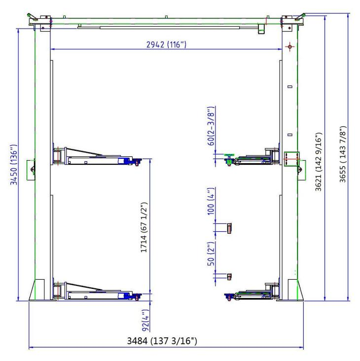
Fig. 1 - Elevation View
