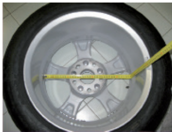
Figure F3.3.1 Example of manual measuring of the external diameter (da2) of the wheel in the ALS1/ ALS2 Programme Type
