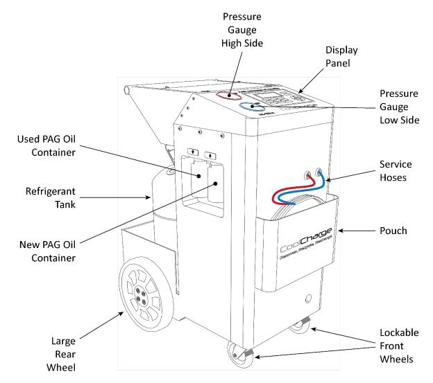
Components on the rear of the AC-134a include:
