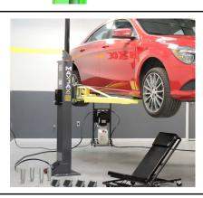
A gunmetal gray powder coat is used that has a significantly lower coefficient of friction than the textured black paint featured on previous Dannmar M6 models. There is evidence that the textured paint had contributed to carriage binding problems on past units.
