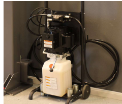
Dual hose storage hooks hung the hoses during storage. Cluttered and messy.
