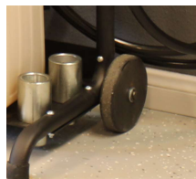
Hard, non-bearing nylon wheels did not roll well over rough surfaces.
