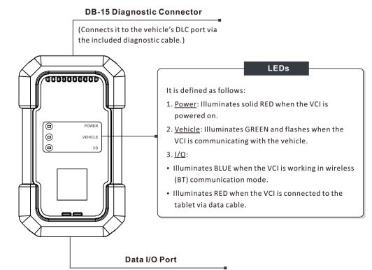
(Connects it to the tablet to perform vehicle diagnosis via the data cable.)
