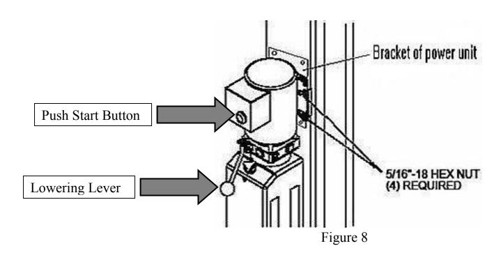
After the securing the power unit to the column, remove the black breather cap and fill the reservoir with approx. 4.5 gallons (18 liters) of ISO-32 hydraulic oil (10 weight hydraulic oil) DO NOT USE TRANSMISSION FLUID or reclaimed hydraulic oil. Use of transmission fluid or reclaimed hydraulic oil will void the manufacturer's warranty.
