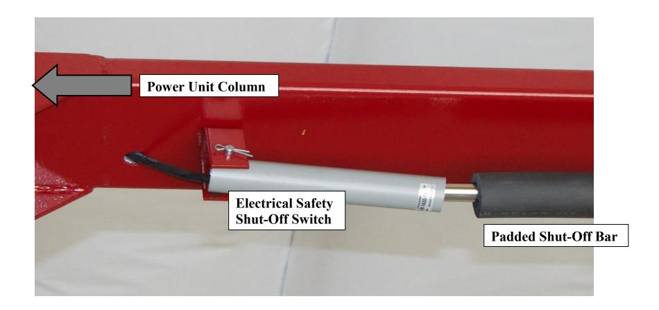
After inserting the rounded end of the shut off bar into the electrical switch (as shown above) connect the flatted end of the padded shut off bar to the underside of the overhead beam adjacent to the slave side column using the provided should bolt and nut. See *photo below for reference*.
