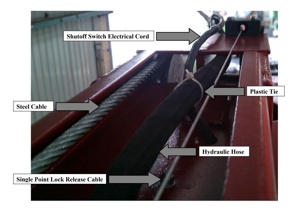
The electrical cord will route over the outer edge of the overhead beam as shown above and downward to the power unit junction box.
