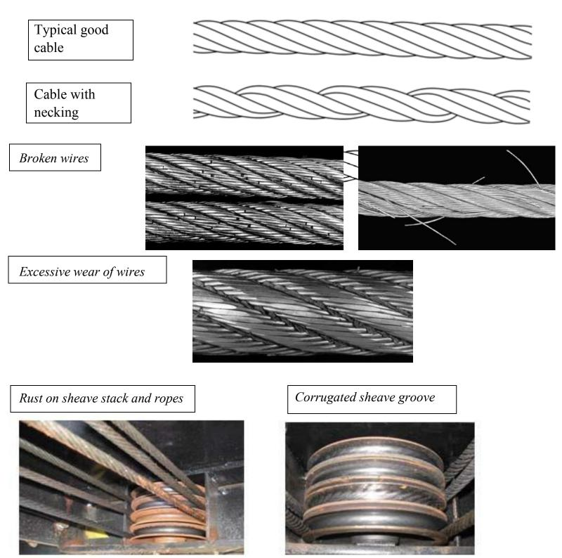
(Pictures above are of a 4-Post Lift, conditions still apply to 2-Post Lifts)
