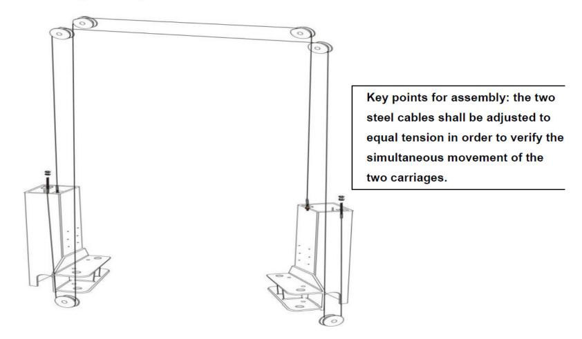
Figure 21: Equalizing Cable Installation
