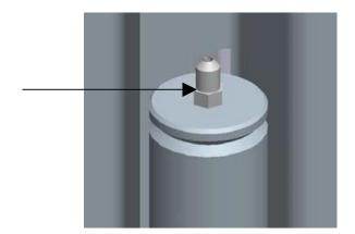
Power up 2"-3". You should hear air escaping around the bleeder valve. Repeat 3-4 times or until only oil is coming out of the bleeder valve.
