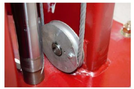
Figure 22: Lower Pulley install
