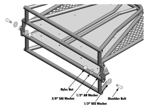
The nuts will tighten down and bottom out on the shoulder bolts. The nuts have "nyloc" and do not require any thread locker. Make sure all hardware is tight.
