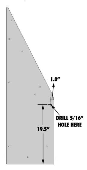
Install the supplied new rubber latch in the location of the drilled hole on the front section of the trailer. Use the hardware from the old latch and tighten.
