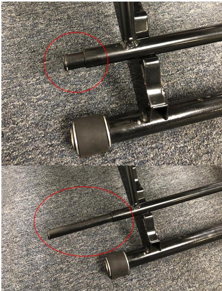
2. Raise the lift slightly (using the hand pump or air compressor) to release the safety bar from its locked position.
