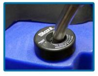
Fill the DEF8000 with new DEF using the cap port on the back of the machine. The tank is capable of holding 30 gallons of new DEF.
