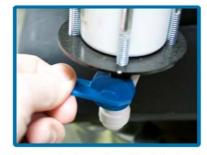
The water bath can be easily drained and refilled using the ball valve at the bottom of the tube. Simply fill the tube with water and open the ball valve to drain it and periodically change the water in the bath.
