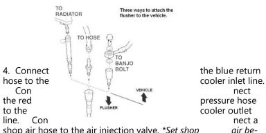
shop air hose to the air injection valve. \*Set shop tween 100-125 psi.
