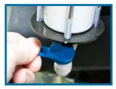
The water bath can be easily drained and refilled using the ball valve at the bottom of the tube. Simply fill the tube with water and open the ball valve to drain it and periodically change the water in the bath.
