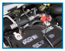
Disconnect red and black battery cables from the vehicle's battery.
