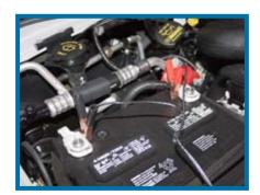
Connect red and black battery cables to vehicle's battery.
