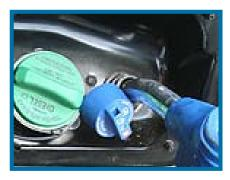
Using the nozzle, fill the vehicle's DEF reservoir with new DEF fluid. The nozzle has a built in vacuum shut off feature that will shut off the flow of DEF when the vehicle's reservoir is full.
