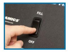
Return switch on the front panel of the machine to the "OFF" position.
