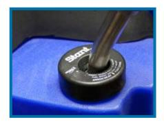
Fill the DEF8000 with new DEF using the cap port on the back of the machine. The tank is capable of holding 30 gallons of new DEF.
