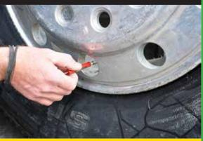
Remove Valve Core to Release Air From Tire Completely.
