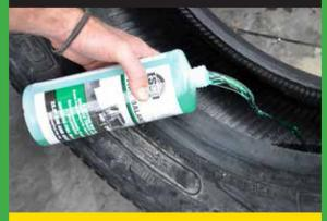
Liquid Tire Balance Can Also Be Installed
