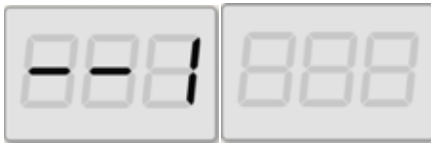
Fig. 23: Search for the balancing planes: the left display indicates to move the sensor forward (move it to the right) to find the exact internal position of the balancing planes
