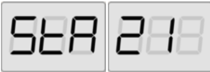
Fig.21: Static imbalance display enabled. The right display indicates the entity of the static imbalance
