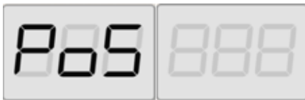
Fig. 25: Search for the balancing planes: the left display indicates that the sensor is exactly on the internal balancing plane
