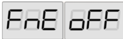
Fig. 29: Disabling imbalance display in high resolution
