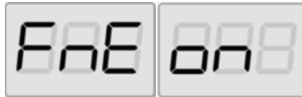
Fig. 28: Enabling imbalance display in high resolution
