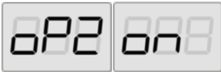
Fig. 30: Enabling operator 2 memory Operator 1 memory is kept
