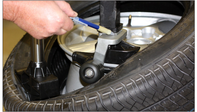
Figure 22 - Duckhead Roller Properly Mounted On Bracket
