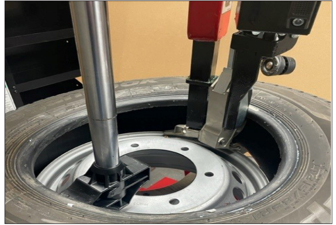
Figure 54 - Push Control Handle Up To Lift Bead Over Rim
