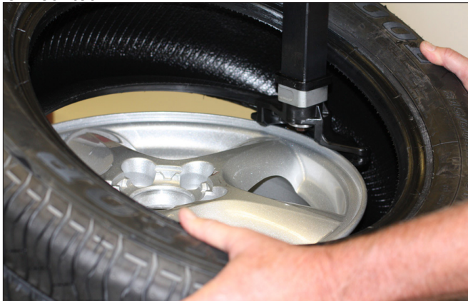
Figure 20 - Mounting Lower Bead
