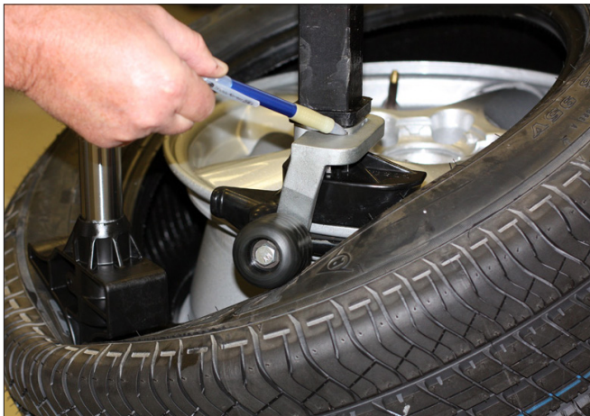
Figure 44 - Duckhead Roller Properly Mounted On Bracket
