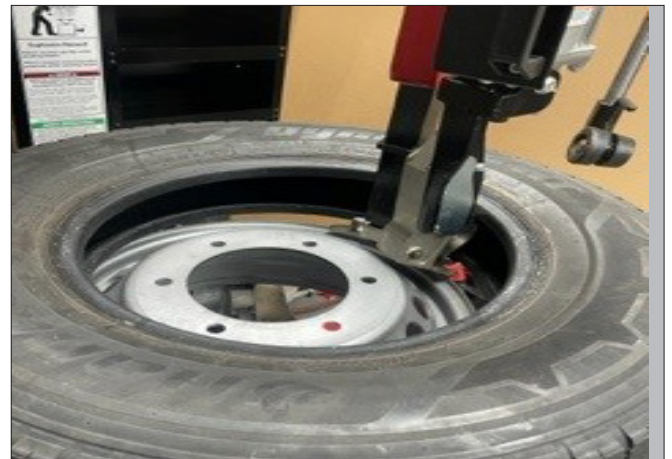
Figure 55 - Demount Lower Tire Bead
