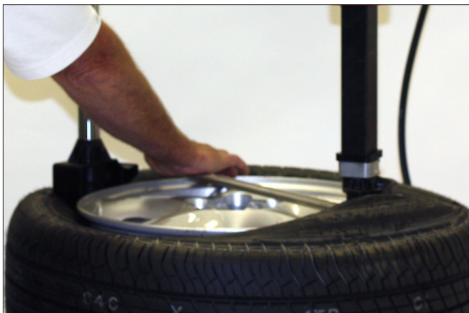
Figure 39 - Rotate Lifting Tool Down for Demount
