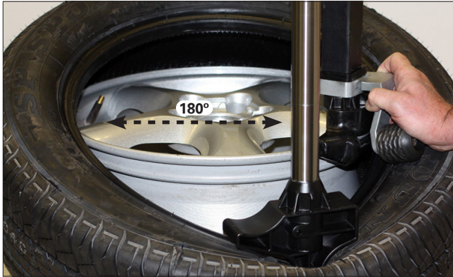
Figure 43 - Position Valve Stem 180° Ahead of Mount/Demount Tool
