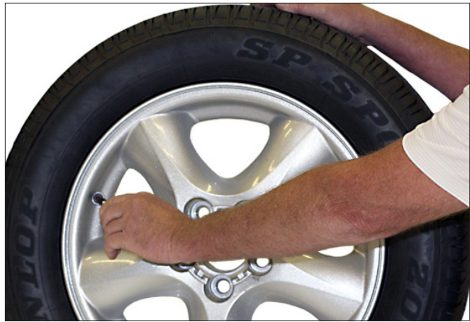
Figure 1 - Remove Valve Core to Deflate Tire
