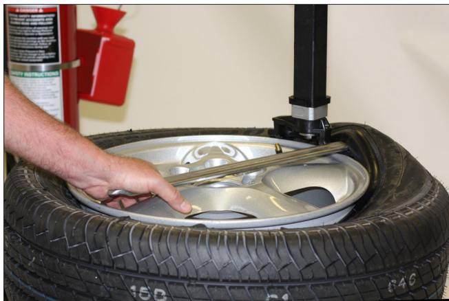
Figure 40 - Rotate Lifting Tool Down for Demount
