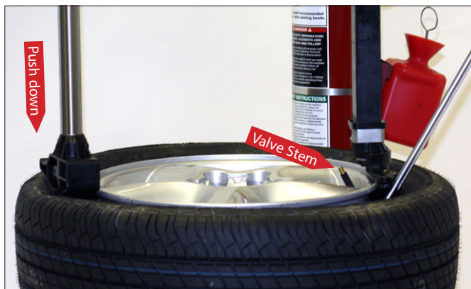
Figure 12 - Insert Bead Lifting Tool
