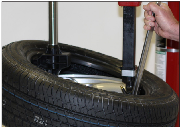
Figure 14 - Demounting Lower Bead
