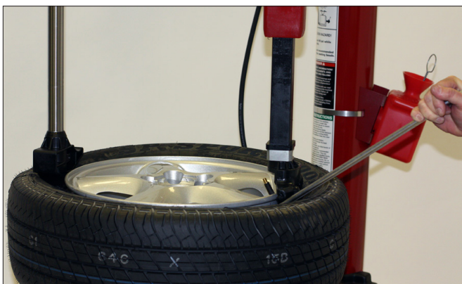
Figure 38 - Helper Foot Pushing Bead Into Drop Center
