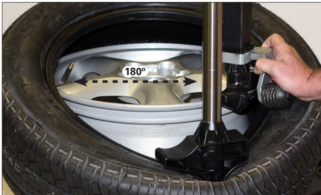
Figure 21 - Position Valve Stem 180° Ahead of Mount Tool
