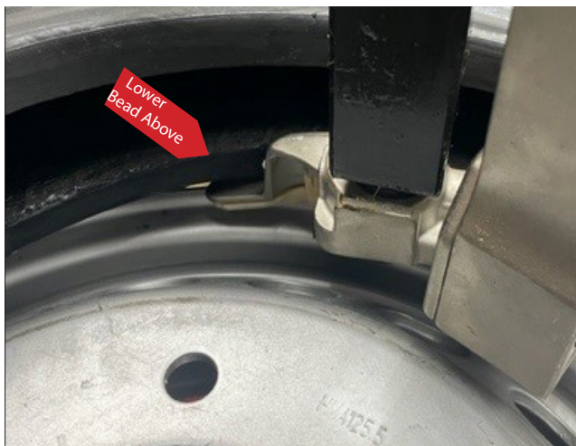
Figure 60 - Robo-Arm and Robo-Roller Pushing Tire Bead in to the Drop Center
