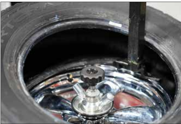
Figure 24 - Mounting Lower Bead
