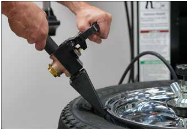
Figure 28 - If Necessary, Use ABS for Bead Sealing
