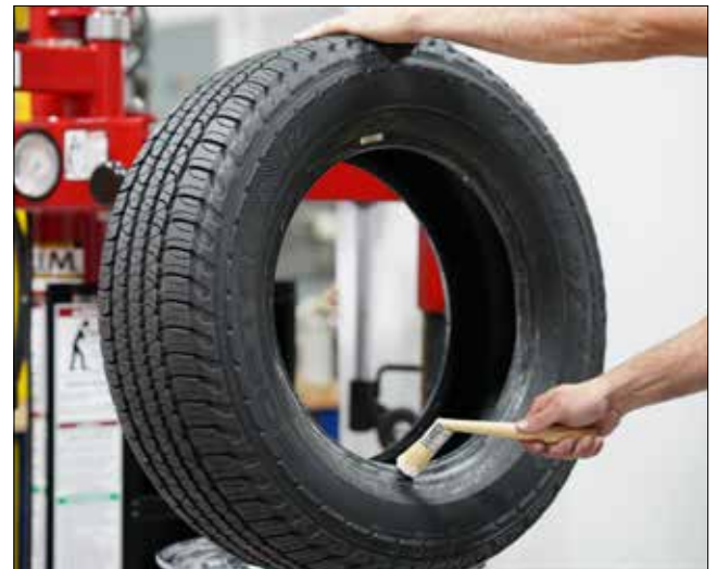
Figure 22 - Lubricate Tire Beads Liberally
