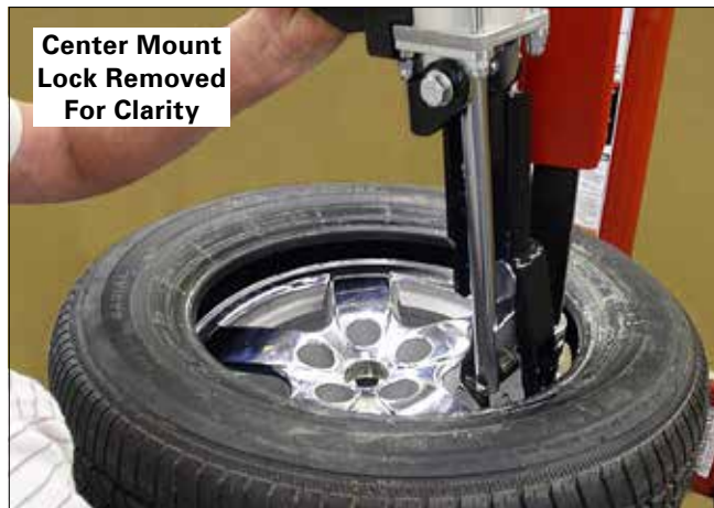
Figure 54 - Push Control Handle Up To Lift Bead Over Rim
