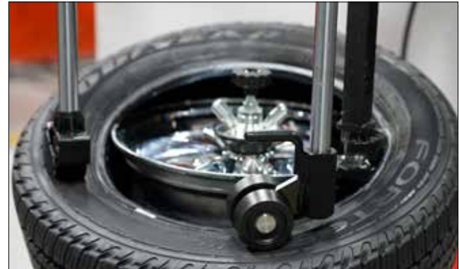
Figure 26 - Mounting Top Bead
