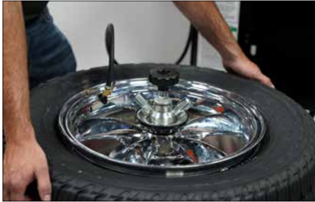
Figure 27 - Lift Tire Upwards for Bead Sealing
