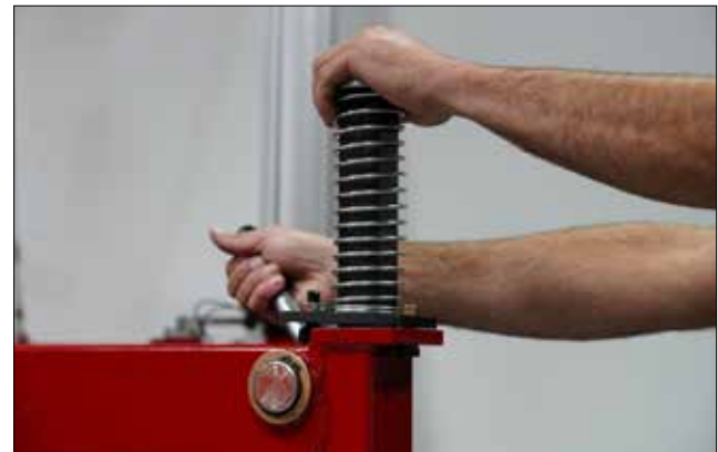
Figure 11 - Position Mount/Demount Tool
