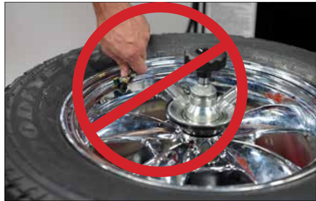
Figure 31 - Do Not Use a Hand-held Style Air Chuck
