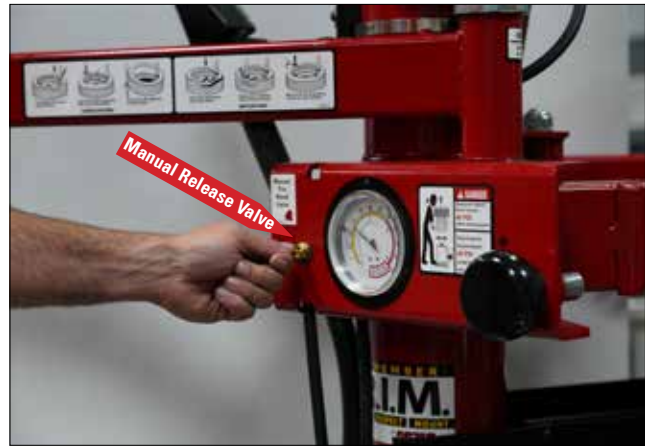
Figure 30 - Location of Manual Release Valve
