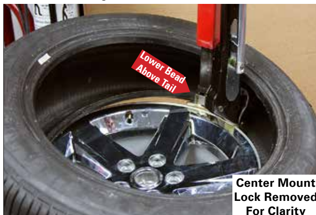
Figure 58 - Position Tire Against Bead Lifter Tool
