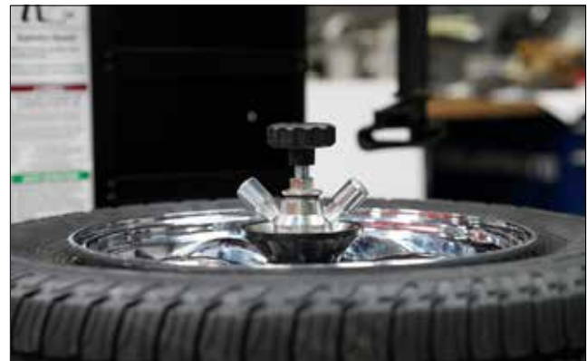
Figure 10 - Tighten Tire/Wheel Assembly to Pedestal
