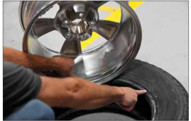
Figure 20 - Verify Size Match Between Tire and Wheel
