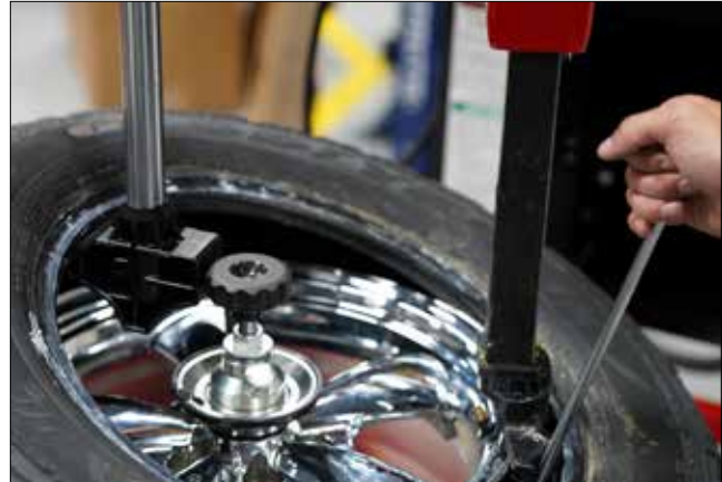
Figure 18 - Demounting Lower Bead
