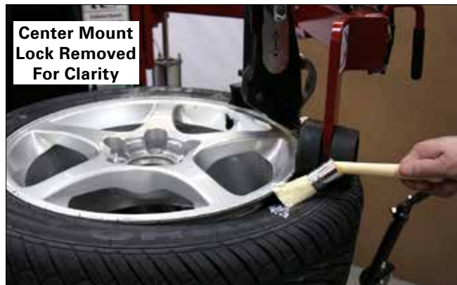
Figure 56 - Use Robo-Roller When Applying Lubricant to Tire Bead
