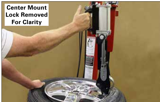
Figure 51 - Leverless Tool Hooked Under Tire Bead
