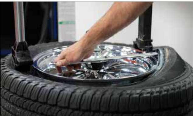
Figure 17 - Lift Bead Over Demount Tool
