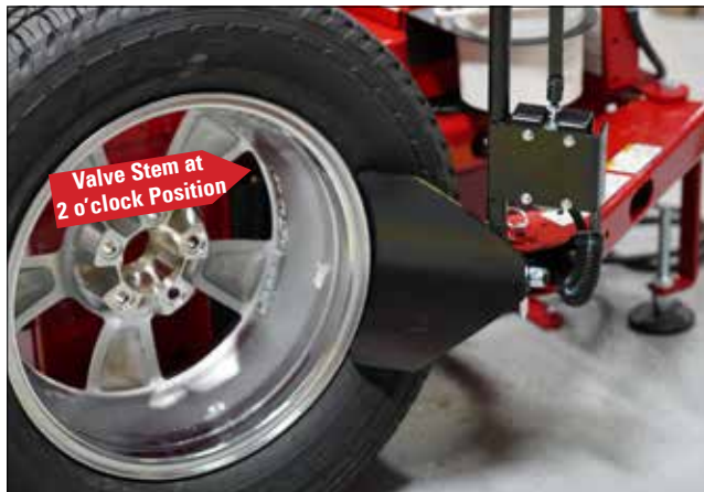
Figure 4 - Position Tire and Bead Loosener Shoe With Wheel Turned Around and Valve Stem in 2 o'clock Position.
