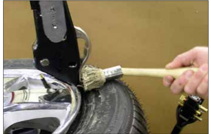
Figure 49 - Apply lubricant to Bead Lifter Tool Hook
