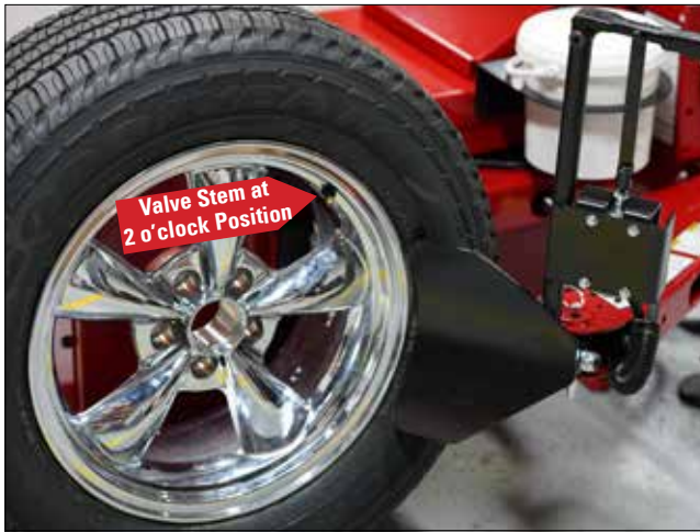
Figure 3 - Position Tire and Bead Loosener Shoe with Valve Stem in 2 o'clock Position.
