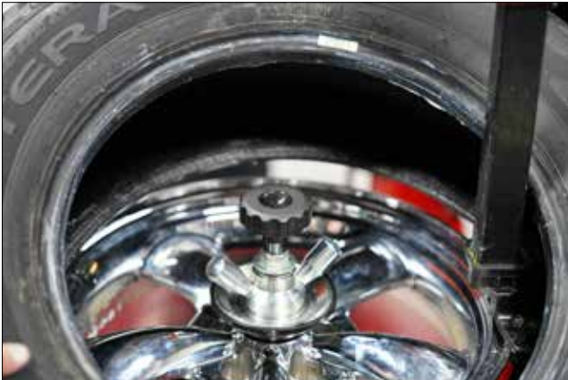
Figure 23 - Position Tire Against Mount/Demount Tool
