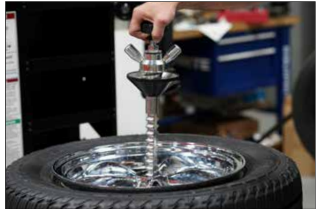
Figure 9 - Place Center Mount Lock through Wheel Center
