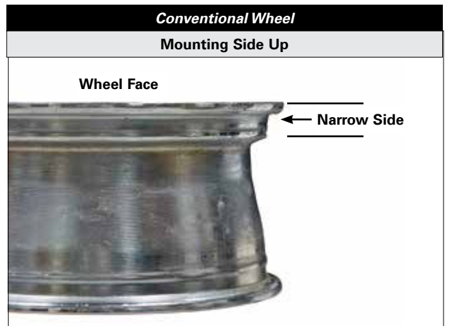
Figure 7a - Mounting Side Up, Conventional Wheel
