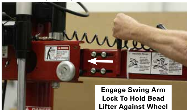
Figure 48 - Lock Swing Arm In Position
