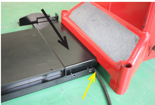
Figure 8 - Bolt PEDAL BOX ASSY to BASE TRACK
