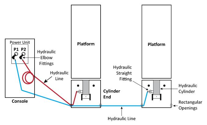
Drawing not to scale. Some components not shown, other components exaggerated for clarity. Fittings shown not connected for clarity.
