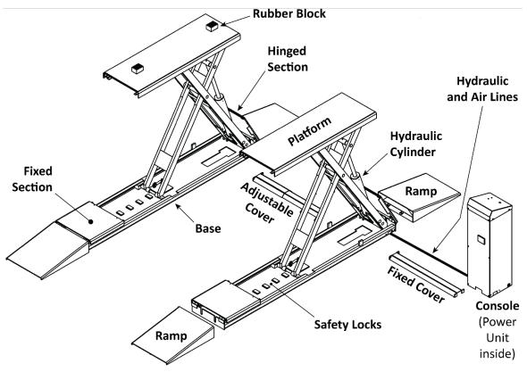
Not necessarily to scale. Not all components shown. The SP-7XL **F** does not have any Ramps.
