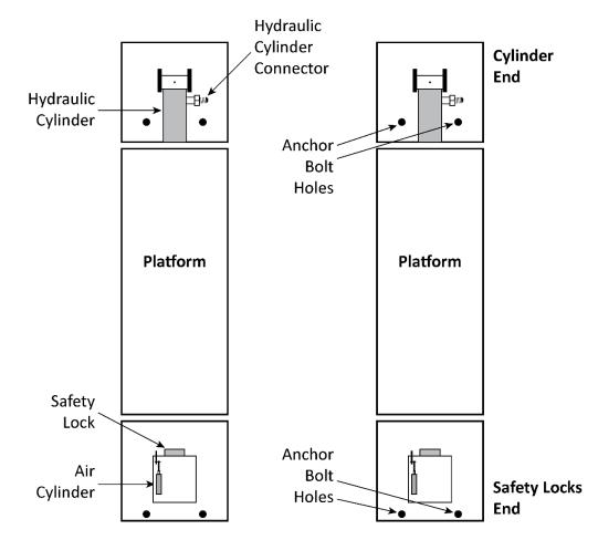
Drawing not necessarily to scale. Not all components shown. Fixed and Hinged Sections shown removed, for clarity.
