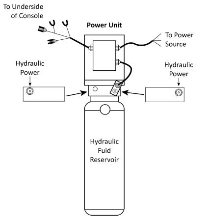
Drawing not necessarily to scale. Not all components shown. Your Power Unit may be slightly different.
