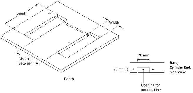
Drawing not necessarily to scale. Not all components shown. There must be 4.25 inches of Concrete **below** the bottom of the Concrete Cutouts. In this drawing, the Console would be on the left (next to where the Length is shown).
