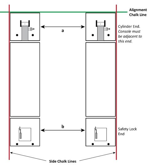
Drawing not necessarily to scale. Not all components shown. Make sure the Console is located adjacent to the Cylinder End of the Lift, not the Safety Lock End.
