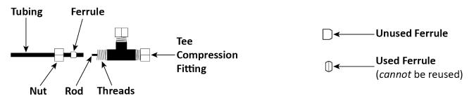
**Important**: *Ferrules can only be tightened once*. When you tighten the Nut on the Threads, the Ferrule gets compressed; it literally changes shape and *cannot* be used again.
