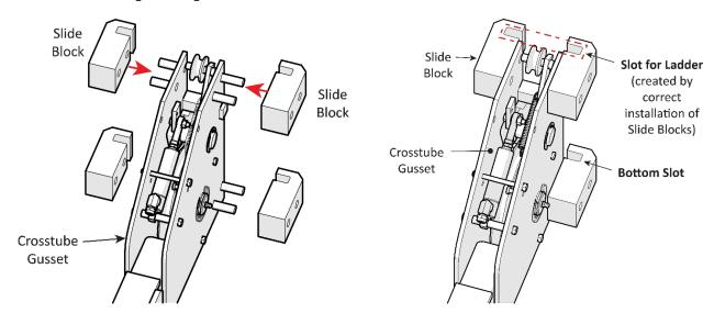
**Important**: It is easy to see the top Slot created by the Slide Blocks. It is difficult to see the bottom Slot, but it is *required* that the Ladder go through *both* Slots.
