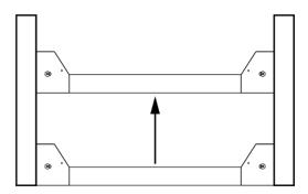
**Important**: The Slack Safety Locks will automatically engage when you raise the Crosstubes. They *cannot* be engaged as you continue with the installation, so *they must be disengaged*.
