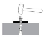
The Expansion Sleeve of the Anchor Bolt may prevent the Anchor Bolt from passing through the hole in the Base Plate too far; this is normal.
