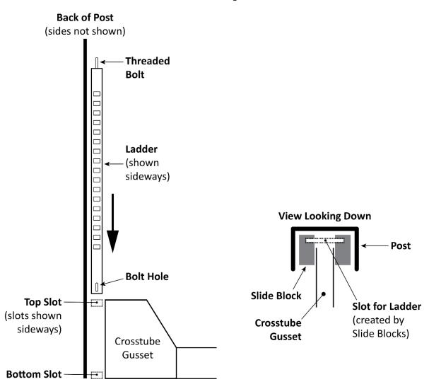
Not to scale. Components removed for clarity. Front and side views combined. Make sure to install each Ladder through **both Slots** on each Crosstube Gusset.
