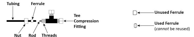
**Important**: *Ferrules can only be tightened once*. When you tighten the Nut on the Threads, the Ferrule is compressed; the Ferrule may not be reused after this compression.
