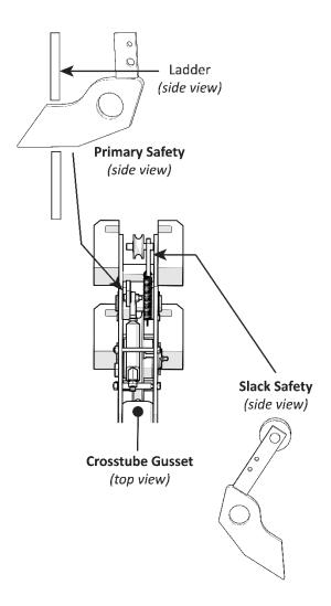
So how do the Runways come down if the Primary Safety Locks are engaged? To lower the Runways, you raise them a few inches (to get them off the Primary Safety Locks), then *press and hold down* the Pushbutton Air Valve. While you hold down the pushbutton, the Primary Safety Locks are moved away from the Safety Lock holes in the Ladders; they are prevented from engaging, which allows the Runways to be lowered.
