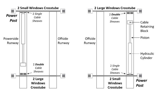
Top view. Drawing not to scale. Components removed for clarity. The location of the Ramps does not change based on Power Post location, but the Power Side Runway and Crosstube locations do. Windows are in the Crosstubes; they are shown here at the ends of the Power Side Runway for clarity.
