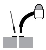
BendPak recommends using a vacuum to get the hole very clean. You can also use a wire brush, hand pump, or compressed air; just *make sure to thoroughly clean each hole*.
