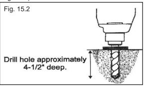
3. After drilling, remove dust thoroughly from each hole using compressed air and/or bristle brush. Make certain that the Columns remain aligned with the chalk line.
