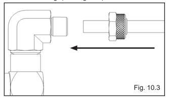
3. Install the 90-degree Hydraulic Fitting in the port at the ram end of the Cylinder. On the pipe thread side of the Fitting it is recommended to use Teflon Tape or pipe sealer. DO NOT USE TEFLON TAPE on the JIC flared end. (See Fig. 10.4)
