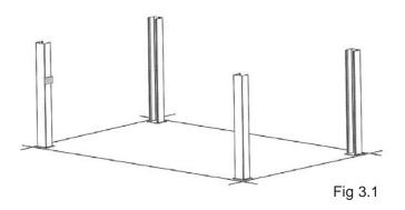
2. To estimate the shim requirements, place a target on floor at each Column position and record the readings. Find the highest of the four locations then find the difference between each of the remaining Columns. This difference is the estimated amount of shim thickness that will be required at each Column. (See Fig. 3.2)
