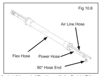
6. Install the end of Flex Hose with the Straight Fitting on the Hydraulic Hose into the hole in the Powerside Runway adjacent to the Power Unit. Install the end of the Flex Hose with the 90° Fitting on the Hydraulic Hose in the Flex Hose Bracket Assy. Tighten the plastic nuts securely. (See Fig 10.7)
