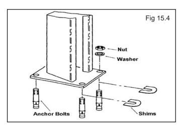
6. After any necessary shims are installed, tighten each nut to 35-45 ft./lbs. IMPORTANT - If Anchor Bolts do not hold when torqued to required amount, concrete must replaced. Saw cut and remove 24" x 24" square area each Column base then re-pour with reinforced 2500 concrete to a depth of six inches minimum, keying new concrete under existing floor. (See Fig. 15.5)
