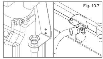
7. Connect the hydraulic hose and air line as shown below making sure the hydraulic hose passes through the retaining rings. MAKE SURE HOSES ARE KEPT CLEAR OF CABLES. There will be one air line hose left unconnected in this step. This air line will be used to activate the pneumatic safety locks in the next step. See page 19 for Compression Fitting instructions. (See Fig. 10.8)
