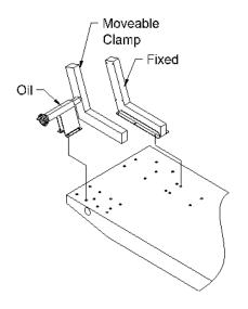
Align two inside hole of the fixed clamp over the existing vise hole pattern as show.
