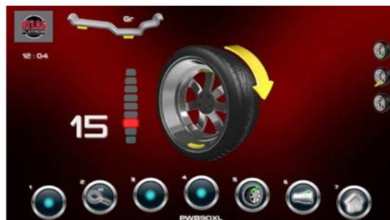
4. At this point, two indications appear on screen for positioning of the imbalance correction weights behind the selected spokes.
