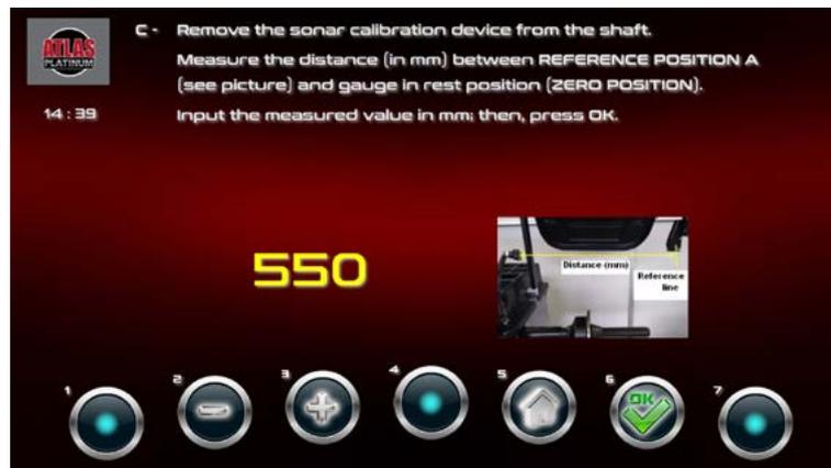
Measure the distance (in mm) between the reference line on the sonar and the distance gauge clip in rest position (ZERO POSITION)
