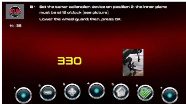
Measure the distance between the reference line on the sonar protection and the plane of the calibration device opposite to the sonar
