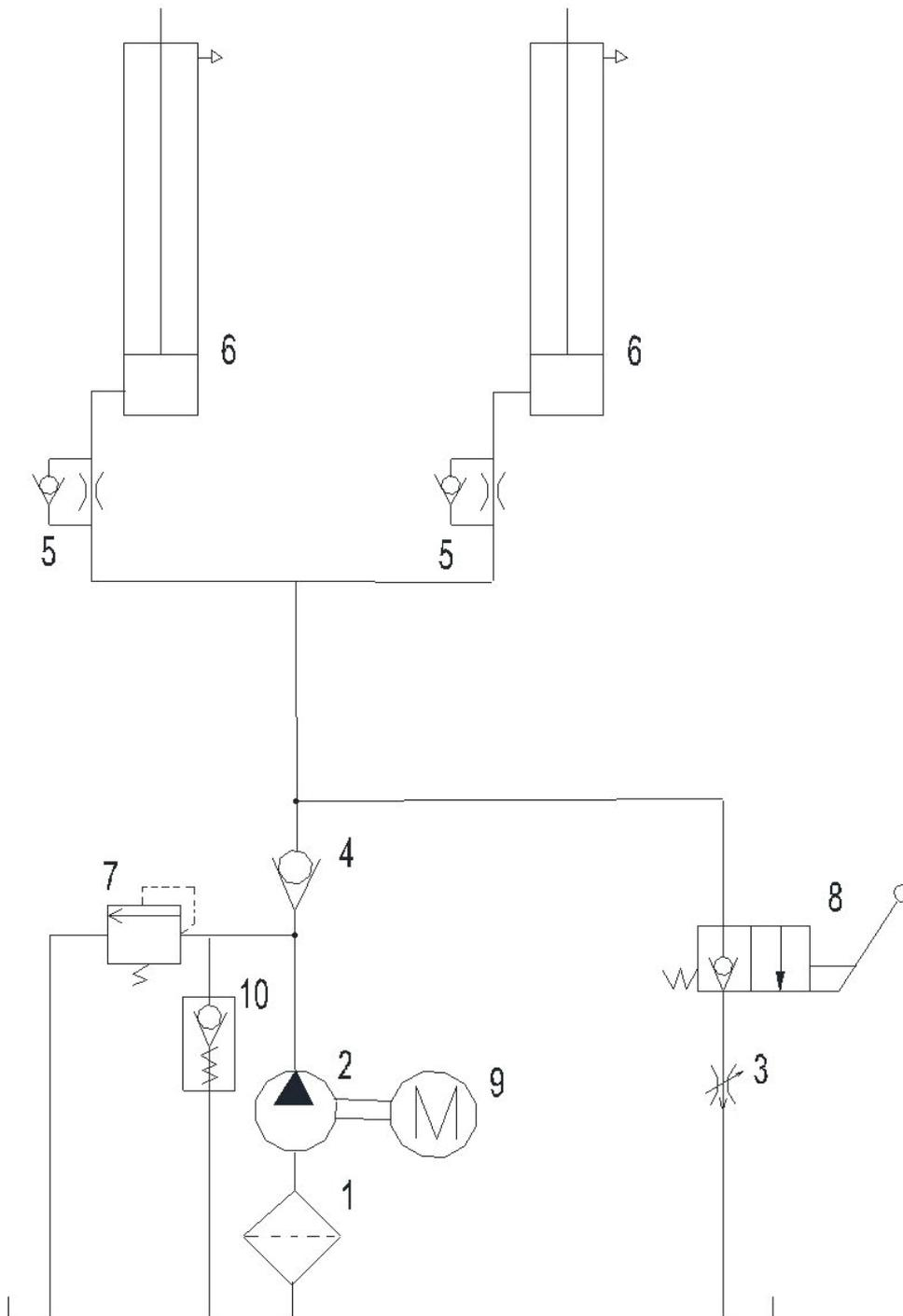
Figure 5 - Hydraulic Plan
