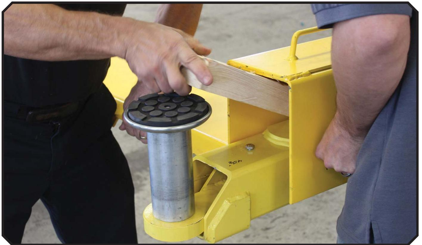
13. Use a level to ensure the Lawn Mower Adapter is resting flat on the lift arms.
