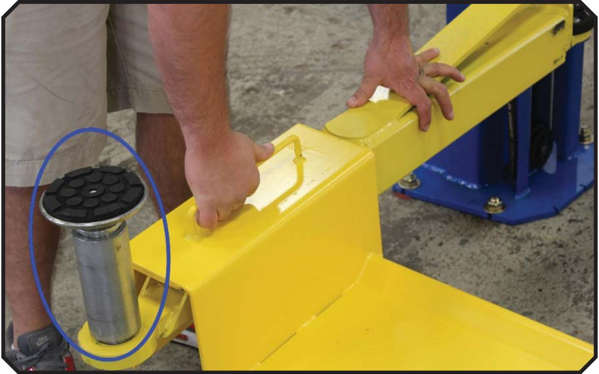
12. If the Lawn Mower Adapter does not sit flat on your lift arms (because all arms vary) then a wood or metal shim may be required to make the Lawn Mower Adapter level.
