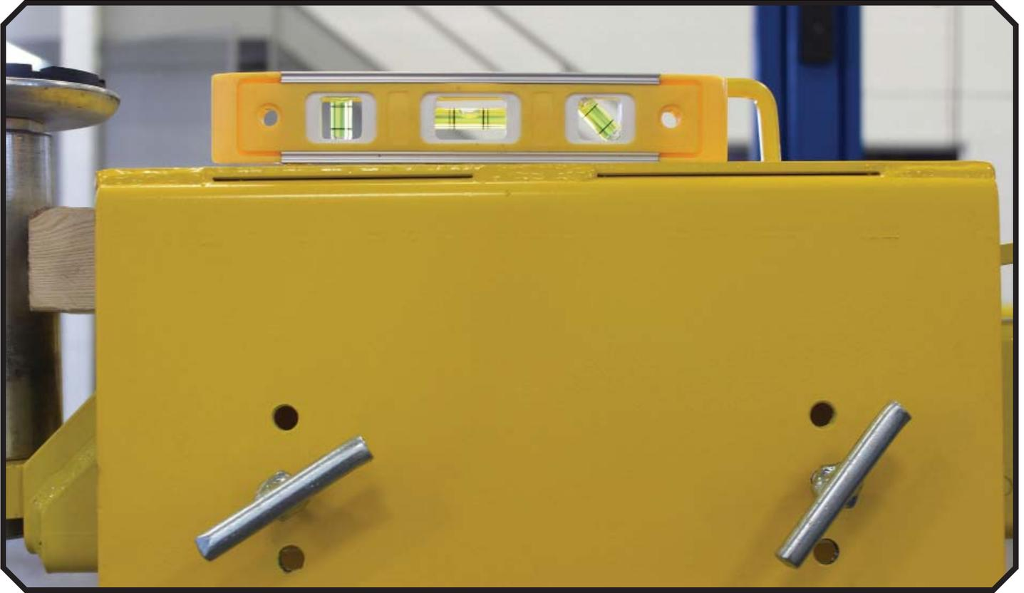
14. Once level, tighten the "T" bolts into the lift arm.
