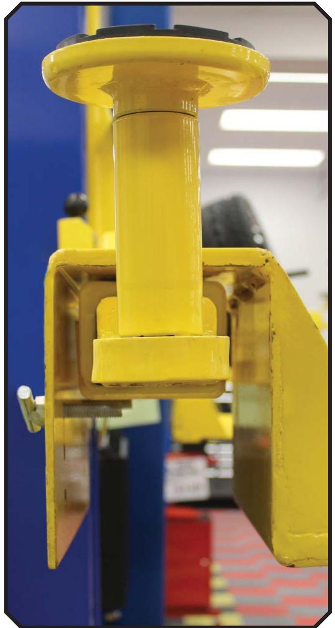
**No shims were needed so the "T" bolt screwed in underneath the lift arm.**
