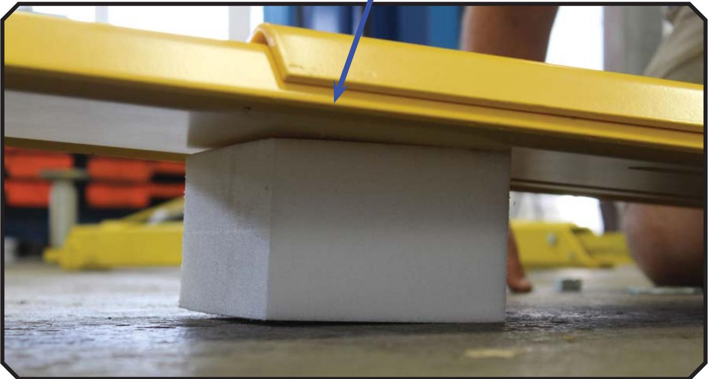
8. Install the hardware. But do not tighten with a wrench until you have the Lawn Mower Adapters on the lift arms.
