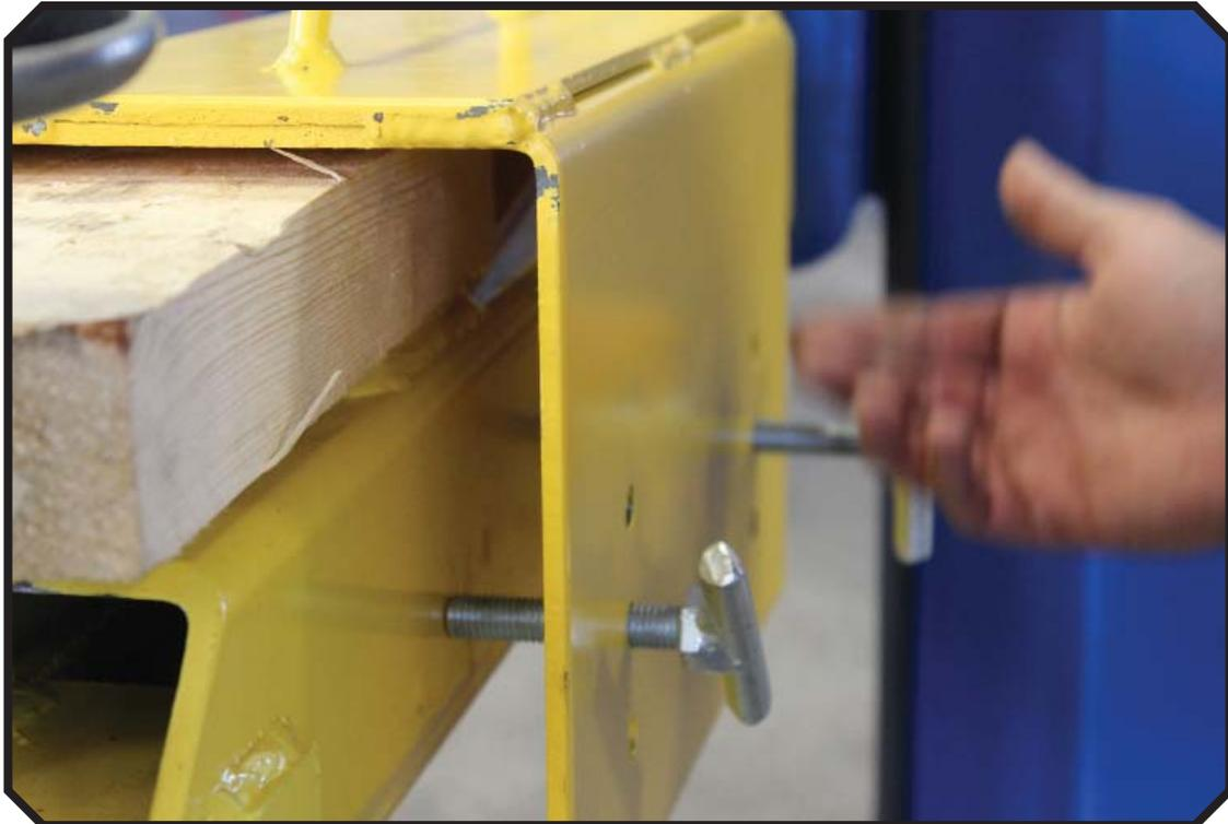
15. If the Lawn Mower Adapter sits flat on the arm without the need for a shim, screw the "T" bolts underneath the arm.
