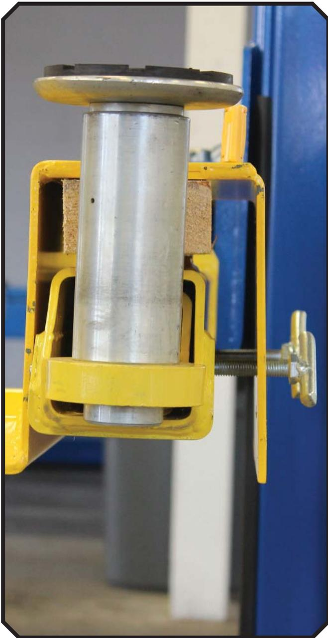
**The shims allowed the "T" bolt to contact the side of the lift arm when screwed in.**
