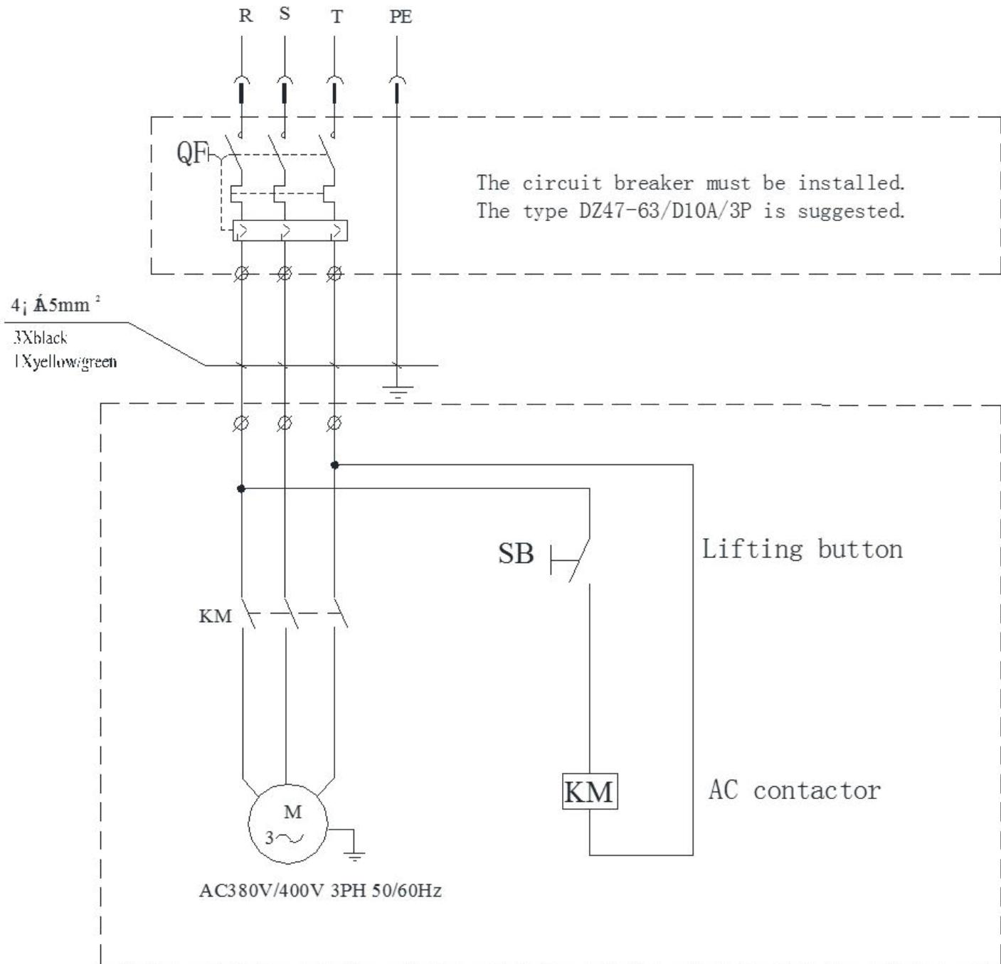
Figure 6b – Electrical Diagram (380V/400V/50Hz/60Hz/3Ph)
