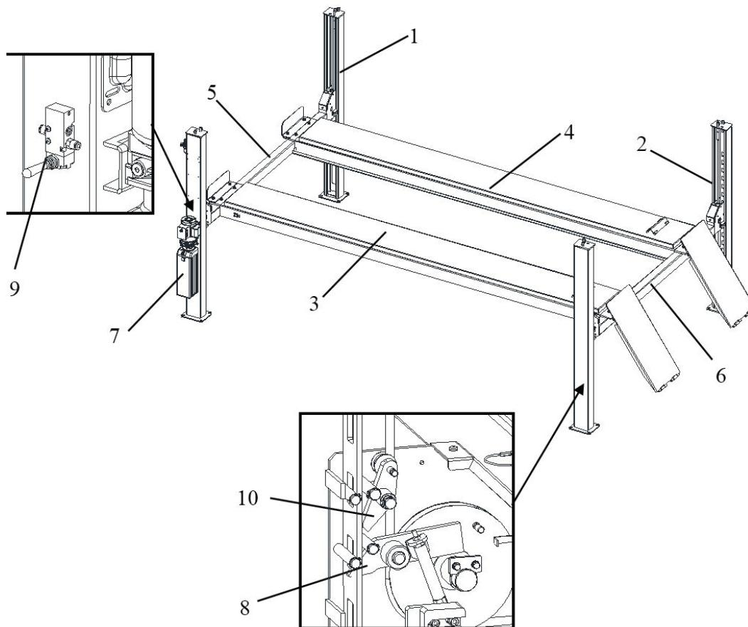
The automatic mechanical back-up safety (8) holds on the lift in the elevated position, can be released by pushing the lever of the control valve (9). The slack cable safety (10) can hold on the lift in event of cable slackening and/or failure.
