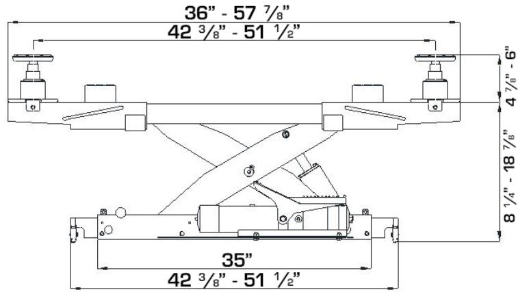
Figure 22 – Jacking Beam Layout
