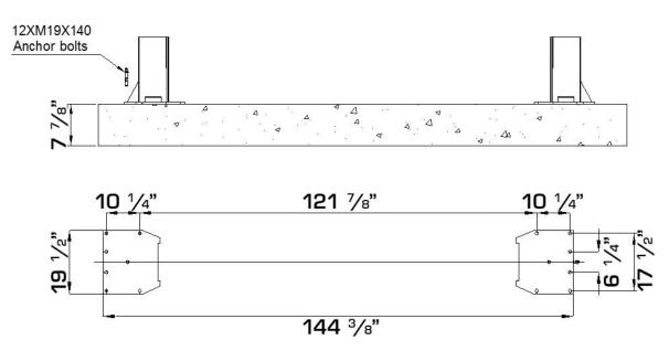
Figure 8 – Floor Plan
