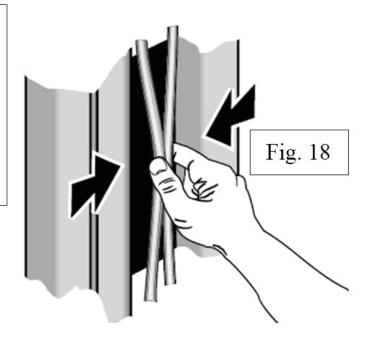
• Adjust the cable tensions if necessary.
