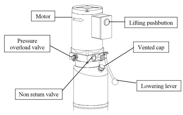
Figure 4 – Hydraulic Power Unit
