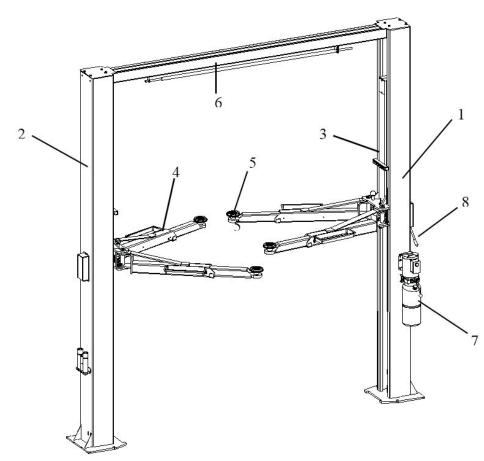
roof. Raising motion is carried out by pushing the lifting button on a power unit (7) which delivers the hydraulic fluid to cylinders inside the columns to act on the chain system to raise the lift. Lowering the vehicle by pushing down the lowering handle on the power unit while holding down the safety lock handle (8).
