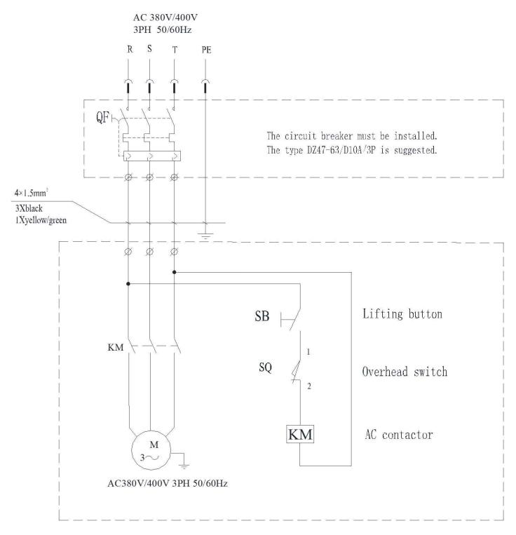
Figure 6b – Electrical Diagram (380V/400V/50Hz/60Hz/3Ph)
