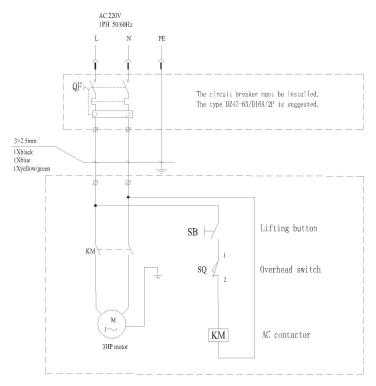
Figure 6a – Electrical Diagram (220V/230V/50Hz/60Hz/1Ph)
