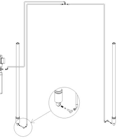
Figure 16 – Hydraulic Line Connection
