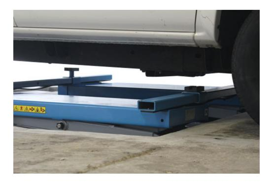
The "higher" the lift can be raised from its fully lowered position (cylinders in a more vertical position) BEFORE it contacts the vehicle's lifting points, will result in greater lifting capacity.
