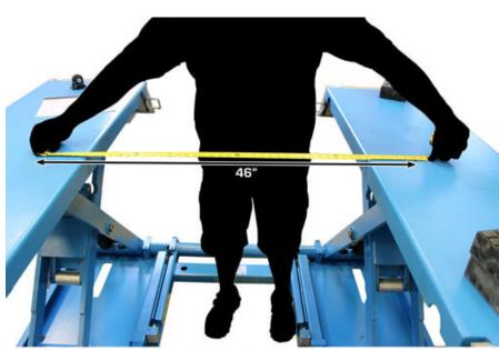
If the lifing points of the vehicle are less than 46" apart (wide), you MUST use cross support bars. (Without support bars, damage may occur)
