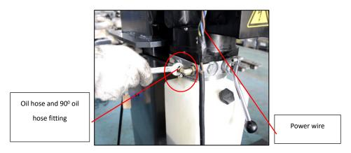
11. Install the oil hose clamp, press with the safety device spring, install the protective cover of safety device and add the hydraulic oil.
