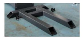
6. Lay the column next to the base and connecting oil hose of cylinder.
