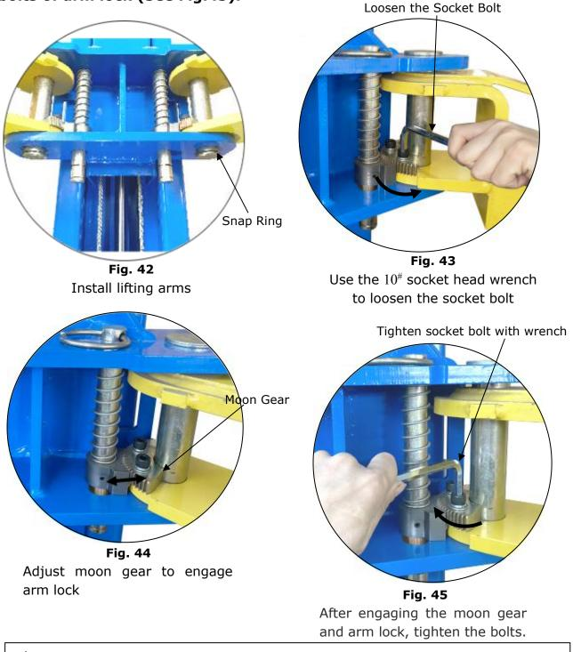
△ DANGER The lift should not be operated until the gears are fully engaged, and it is important to regularly check and adjust the arm restraint gears on all four arms. Failure to do so can result in vehicle damage, injury, or even death.
