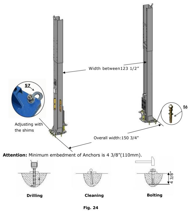
$\triangle$  CAUTION Concrete and anchor bolts must comply with above
