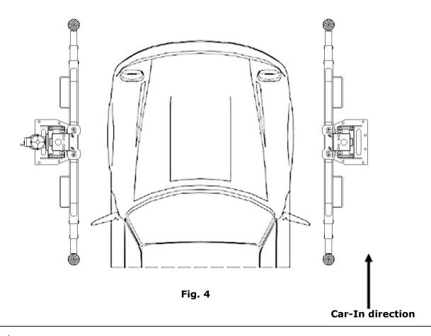
△ CAUTION When driving the vehicle into the lift, ensure that it is positioned in middle of two columns. Any contact with the lift could result in damage to either the vehicle or lift.
