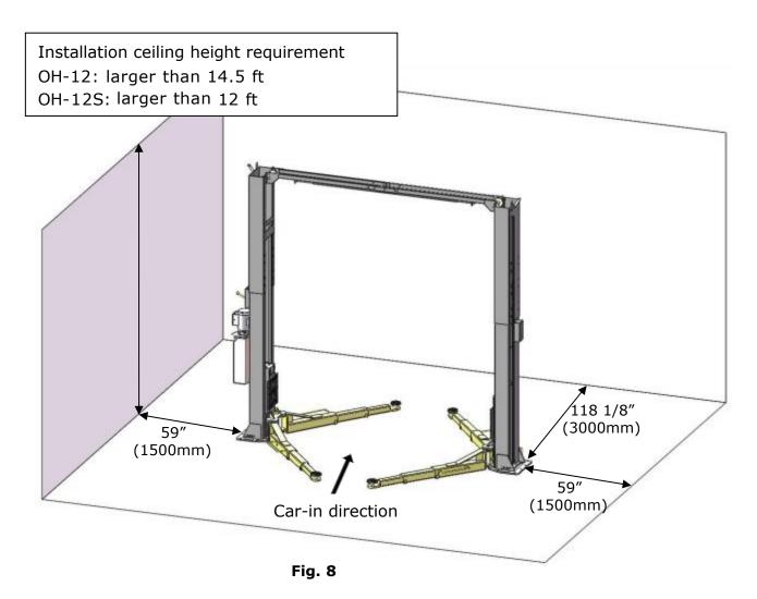
Lift installation and concrete construction must comply with the latest version of the National standard "Automotive Lifts - Safety Requirements for Construction, Testing and Verification". Uniform building codes of other agencies or International Building Codes (IBC) for any special regional structures must meet seismic standards.
