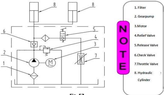
Fig. 57 Hydraulic Schematic Diagram
