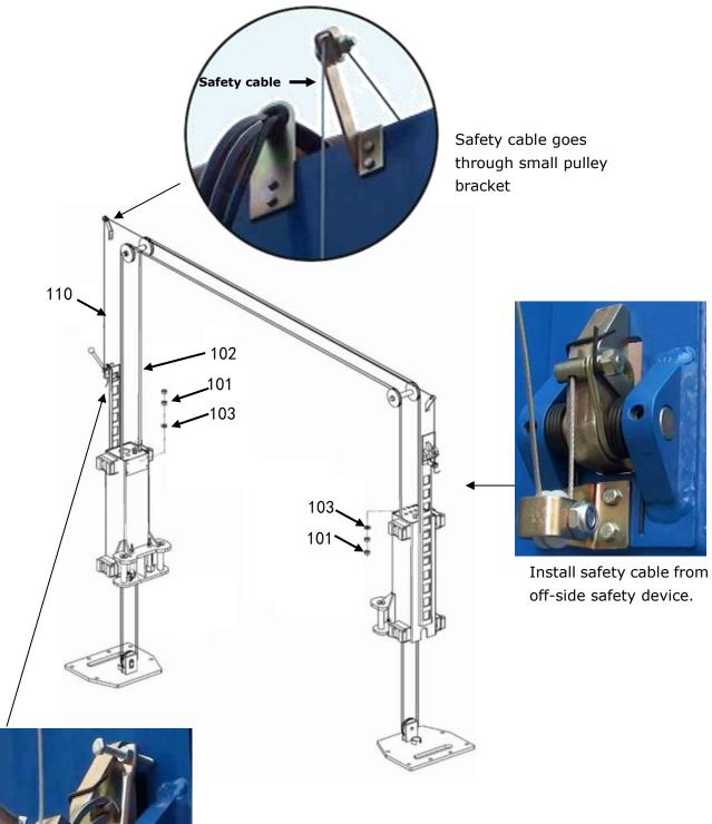
Safety cable is connected with the power-side safety assy.
