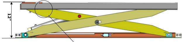
When the lift lowers to 12"(300mm) from ground, the platform touch limit switch road, effect the limit switch to stop lowering. This time press both button DOWN and PASS to lower the lift, along with alarm tone.
