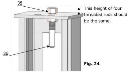
Pass the safety ladder through the hole of the top plate, then tighten the two nuts.
