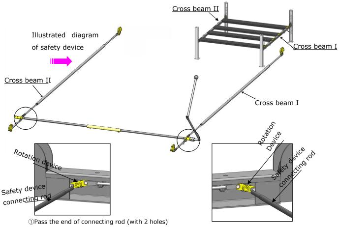
①Pass the end of connecting rod (with 2 holes) through the rotation device of inner side of cross beam II
