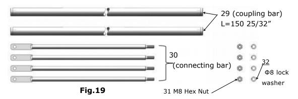
2. Assembly of coupling bar assembly. See fig 20
