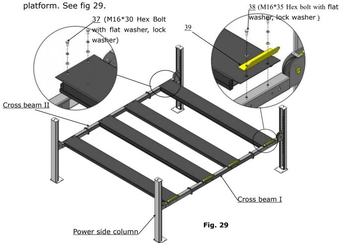
3. Install platform side connecting bolts and cross beam slide blocks. Finally, tighten all the connecting bolts of platform.
