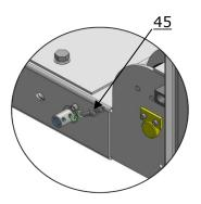
② Align the mounting hole on the outside of cross beam II, tighten with M8\*35 socket bolt with lock washer.
