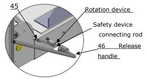
④ Install Release handle on the cross beam I, align the mounting hole, tighten with M8\*35 socket bolt with lock washer.
