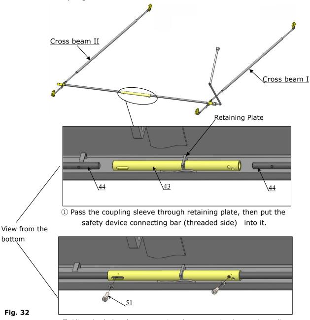
② Align the holes that connecting the connecting bar and coupling sleeve as show above, tighten with M28\*25 socket bolt with lock washer.
