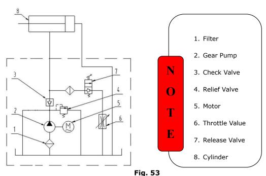
Hydraulic Schematic Diagram
