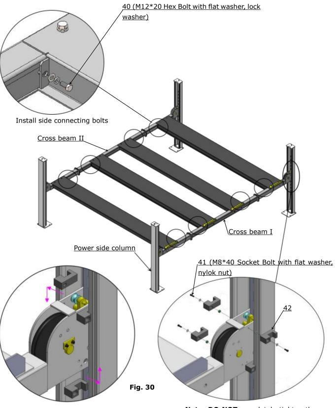
Pass the slide block along the bend edges of column to the gap between column and cross beam. Align to the mounting holes of cross beam and bolt with cross beam.
