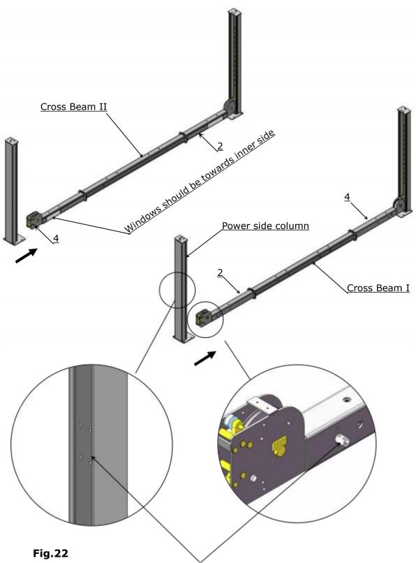
The column with 4- $\Phi$ 10 holes is power side, and rotation device must be towards outside.
