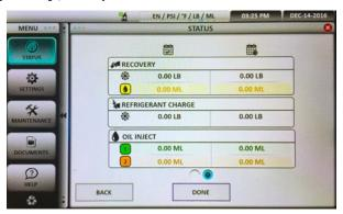
The values on the left side of the screen will display the last amount of recovered refrigerant, refrigerant charged and oil injected. The values on the right side of the screen display the lifetime totals of recovered refrigerant, refrigerant charged and oil injected.
