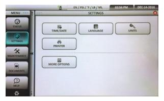
TIME/DATE: To set the time and date press the corresponding up or down arrows. Press
