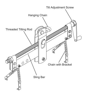
Figure 1 - Engine Sling components
