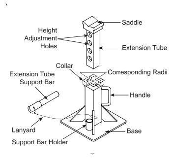
Figure 1 - Model ATD-7449A components
