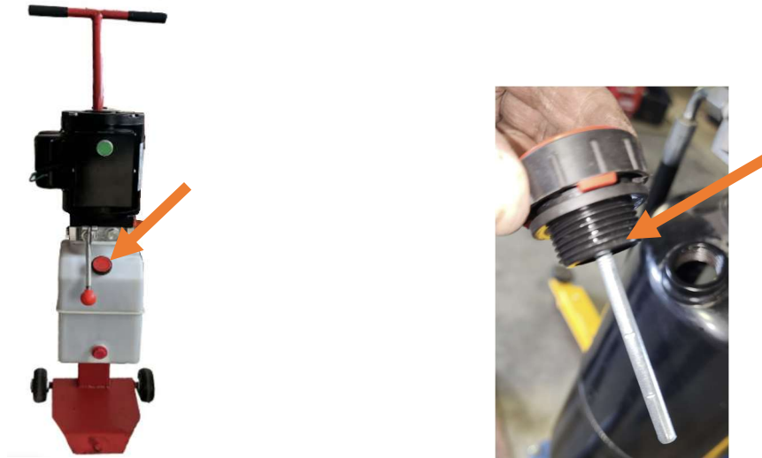
Figure 15: Hydraulic Reservoir Fill Port and Fill Level Mark
