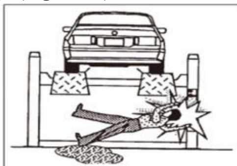
Figure 35 - Slip and fall risk
