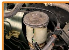
Close ball valve on yellow pressure hose and disconnect hose from master cylinder adapter. Remove the adapter and replace the master cylinder cap.
