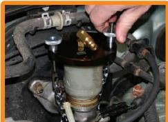
Remove master cylinder cap. Find correct master cylinder adapter from adapter kit and attach to master cylinder reservoir. Connect yellow pressure hose to master cylinder adapter.
