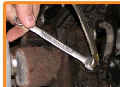
Open the bleeder screw about 1/4 turn until fluid begins to flow into the bottle.
