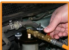
After brake flush is complete, turn the machine off and disconnect the battery cables.
