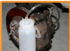
Attach the tube from the used fluid bottle to one of the vehicle's bleeder screws. You may need to verify that the bleeder screw can be opened before attaching the tube. The bottle may be mounted to the caliper using the attached magnet.
