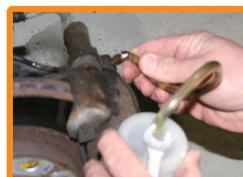
When finished, close the bleeder screw and remove tube from fitting. Repeat process on the remaining three wheels.
