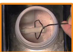
Before draining, bypass the fluid level sensor located in the new fluid tank by pulling up with a wire loop.
