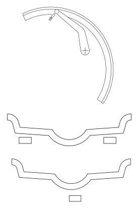
a. Extract the gauge up to the barycentre of the inside correction weight. Use the relative gauge on the machine to measure this.
