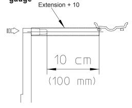
The extension increases the distance measuring range of the gauge by 10 cm.
