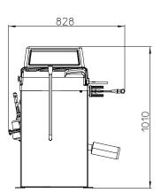
The machine complete with flange weighs 110 kg.
