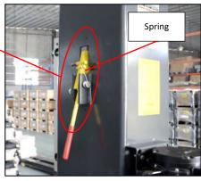
12. Install Supporting arm (left and right) (Rise the lifting platform to first grade of safety lock to make it easier to install)
