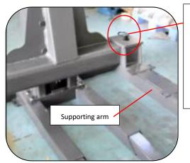
Install the pin and Snap Ring (can use a hammer to help if the pin is too tight)
