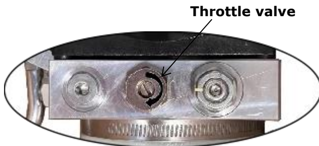
Clockwise to decrease the lowering speed
