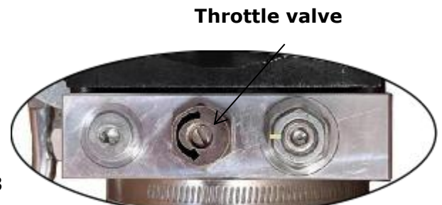
Counterclockwise to increase lowering speed.
