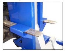
Fig. 4a & 4b Forklift pockets on Column
